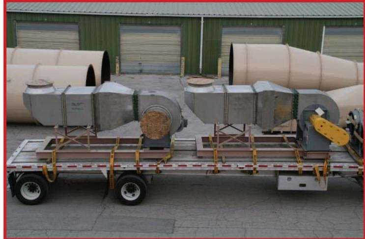
PiTTek has provided Steel Temper Mill and Steel Skin Pass Mills with RME-4 Fume Exhaust Systems. Some features of these systems will vary with the type of mill and the choice of coolant/lubricant used.
